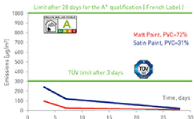
Emission behaviour of optimised interior paints based on VAE-Copolymers
