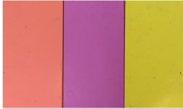
Figure 4 – Vamac® HyPR 5000 series compounds with less staining Naugard® 445, 5phr TiO 2 and 2phr pigment to produce bright colors with good heat ageing
