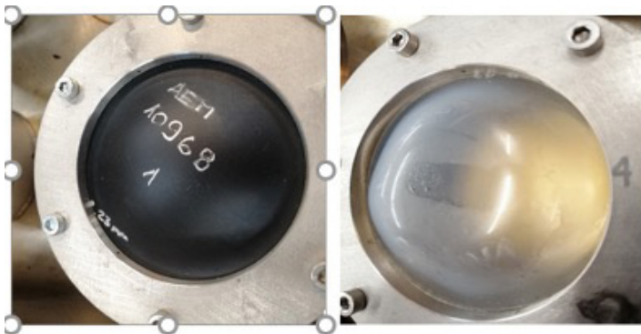
The outer surface of a Vamac® AEM membrane (left) vs. an LSR membrane (right)
