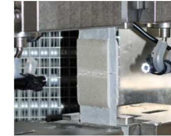
Crack-bridging ability EN 14891 Flexible waterproofing membranes
