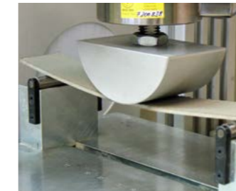
Transverse deformation EN 12004 Tile adhesives
