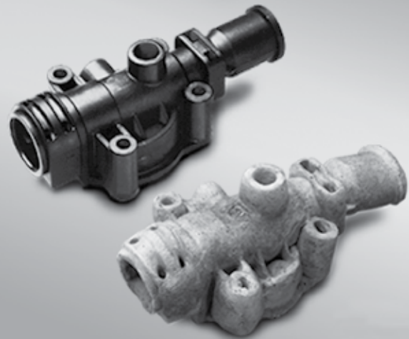
After burning off, a molding (example: pump head made from Celstran PA66-GF50, top) retains its geometry almost intact as a fiber skeleton (bottom)
