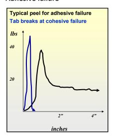
Occurs when bond strength between TPV and engineered thermoplastic is weaker than bulk tensile strength of TPV
