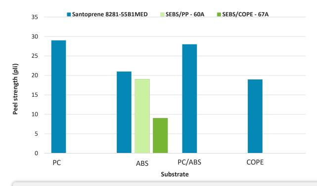
T-bars tested per modified ASTM D1876. Adhesion samples were insert molded @ 257°C (495°F) at 3mm
