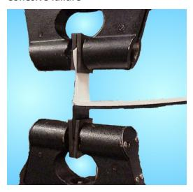
Occurs when bond strength between the TPV and engineered thermoplastic\* substrate exceeds bulk tensile strength of TPV
