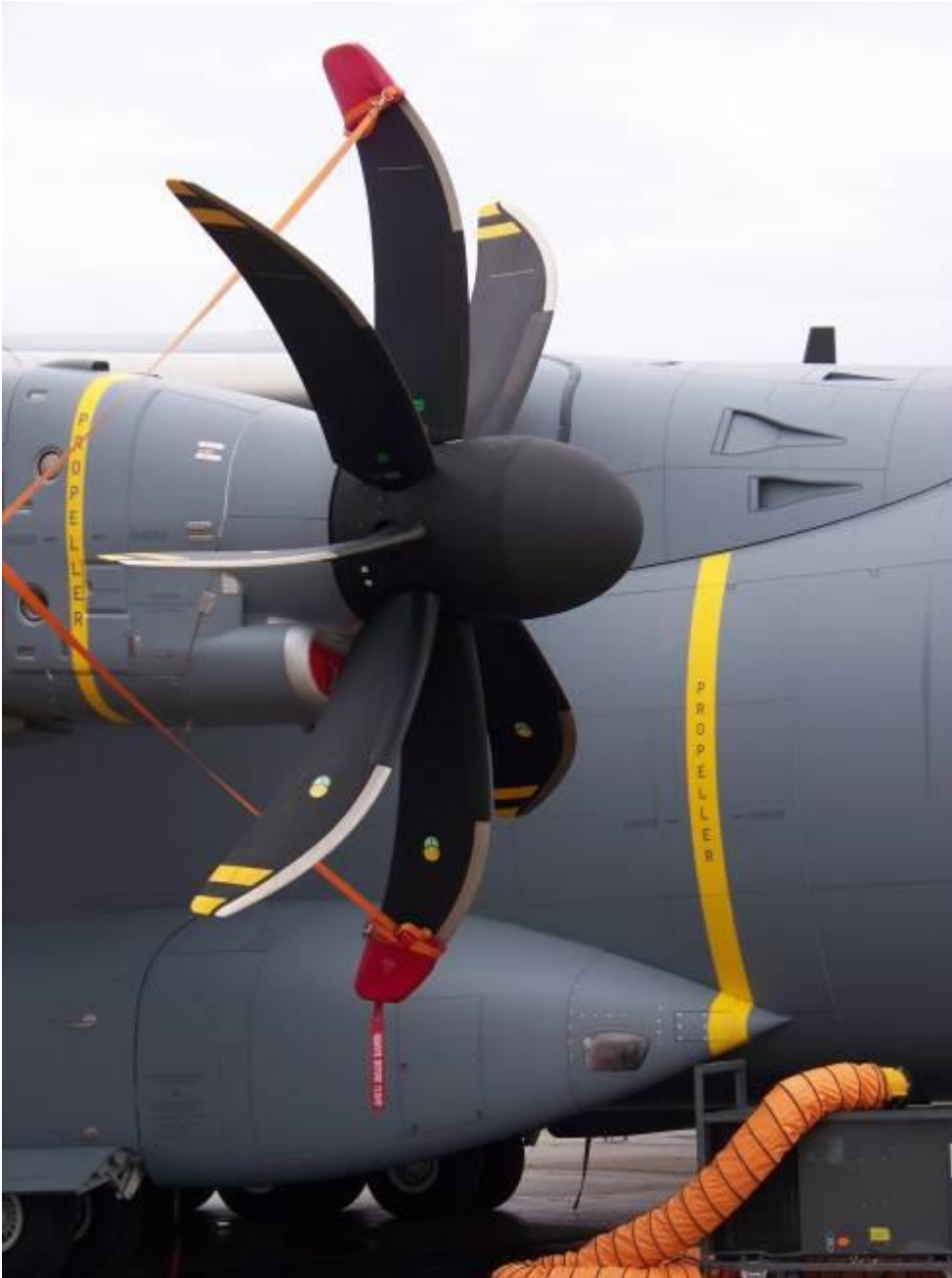
Excellent Impact Resistance — New Airbus A400M military transport aircraft feature fuselage ice protection plates made with glass fabric-based Fortron ® polyphenylene sulfide (PPS) from Celanese. Photo copyright A. Offringa, Fokker Aerostructures
