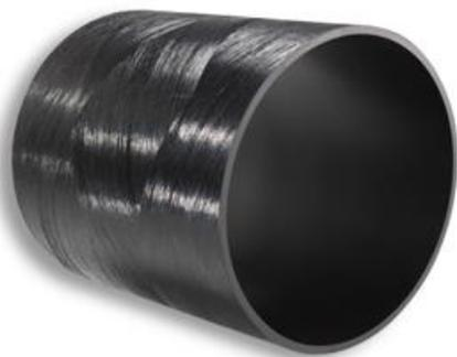
**2013 Oil & Gas Award Winner** — Innovative Fiberflex<sup>®</sup>-11 pipe from Composite Fluid Transfer incorporates Celstran<sup>®</sup> CFR-TP continuous fiberglass reinforced high-density polyethylene (HDPE) thermoplastic composite tape from Celanese, which is wound around and heat consolidated to a specially designed, extruded thin-wall HDPE thermoplastic liner.
