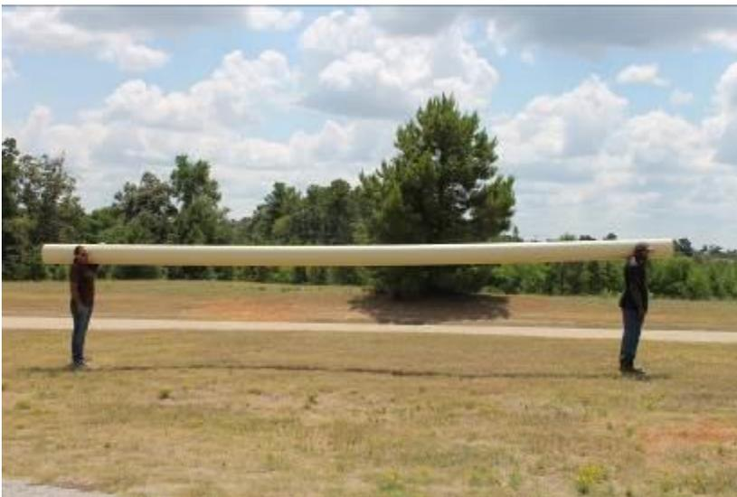
**Easy to Lift** — Two people in the field can easily lift and carry a 30-foot section of Fiberflex<sup>®</sup>-11 pipe that features Celstran<sup>®</sup> continuous fiber reinforced thermoplastic composites (CFR-TP) from Celanese.
