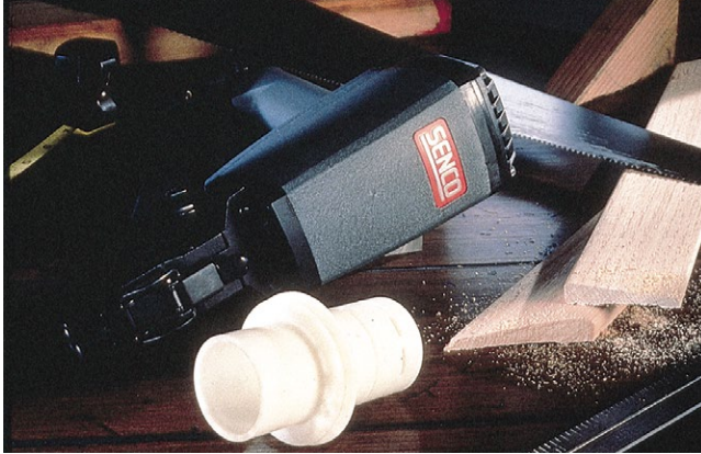
By switching from aluminum to Celcon® acetal copolymer, Senco Products, Inc. was able to produce longer lasting drive cylinders at a lower cost.
