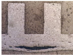
Cross section of blistering sample (connector housing)
