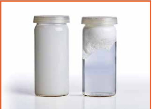
GUR® UHMW-PE is inherently hydrophobic: the GUR® UHMW-PE powder does not mix with water and floats on the surface. (right side). However, Celanese offers as well hydrophilic grades, which mix well with water (left side)
