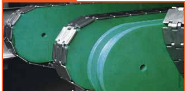
Chain guide, typical application for GUR® UHMW-PE.
