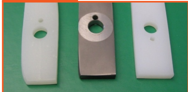
Test specimens of Sand-Slurry Test: GUR® UHMW-PE (on the right) shows the lowest abrasion values, compared to HDPE (left) and steel (middle).
