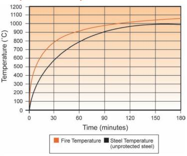
Unprotected steel weakens when exposed to temperatures above 500°C. Under conditions of a typical fire, it can reach this critical temperature in approximately 20 minutes, resulting in instability and risk of complete collapse.
