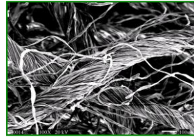
8-Ply, woven cotton at 100x magnification
