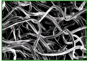
Celaire™ non-woven at 100x magnification
